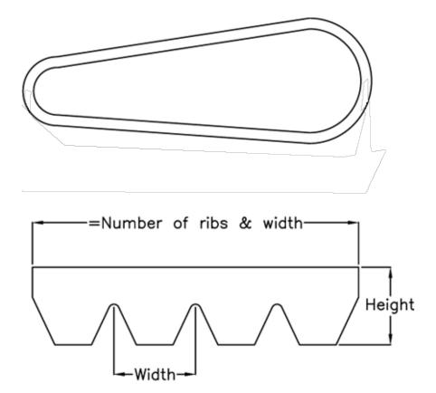
$\begin{array}{ll} \text{Datum Llength} = 6883 \\ \text{Height} &= 16.5 \\ \text{Number of ribs} = 6 \\ \text{Pitch} &= 9.4 \end{array}$
